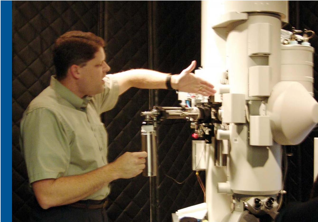
with two cryoelectron microscopes, which are capable of helping scientists see biological structures that are too small for conventional electron microscopy and too large to be resolved by X-ray crystallography. The facility now also has all the equipment needed to handle thick specimens, which are fundamental in studying large cells and tissues.
